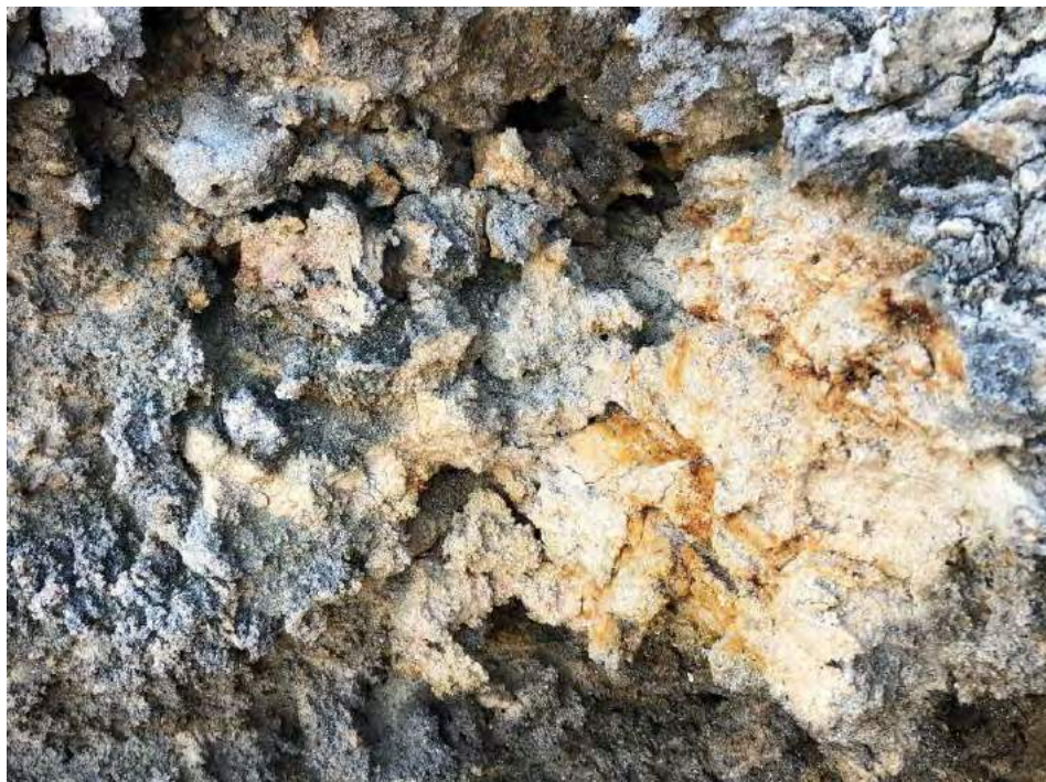
Highly leached and friable rock mass. Yellow colouration indicates materials has recently broken away from cliff
