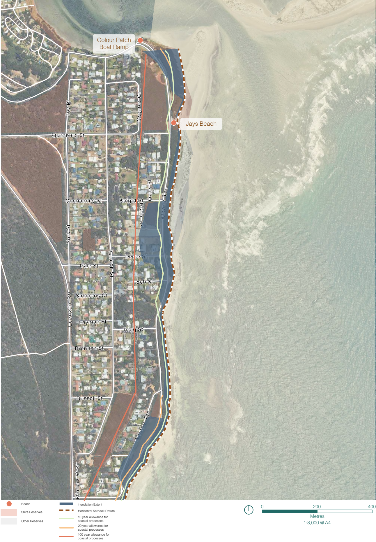
FIGURE 2.12 - HAZARD LINES AND INUNDATION AREAS - AUGUSTA NORTH
