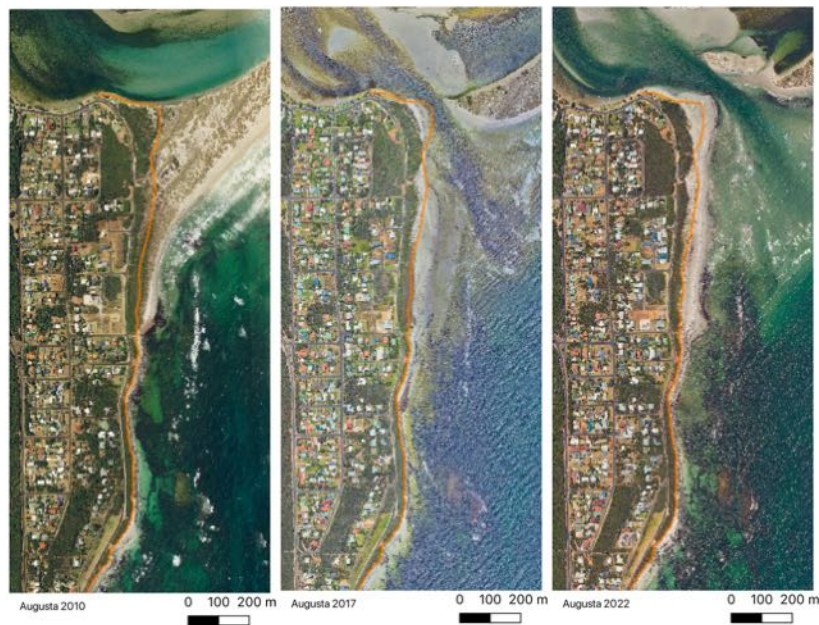
Figure 4-6 Aerial imagery showing August Blackwood Rivermouth Dynamics in 2010 (prior to new alignment), and changes in the past five years from 2017 to 2022.
