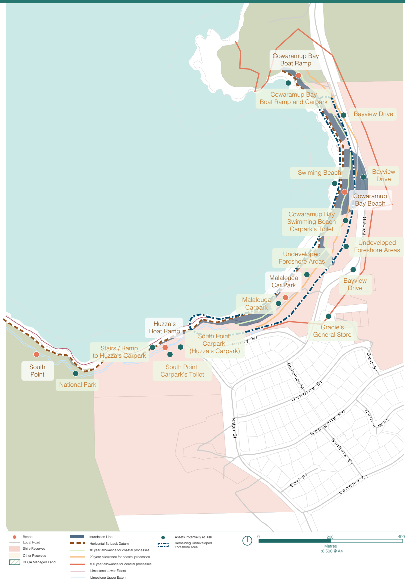
FIGURE 3.1 – GRACETOWN HAZARD LINES, INUNDATION AREAS AND ASSETS
