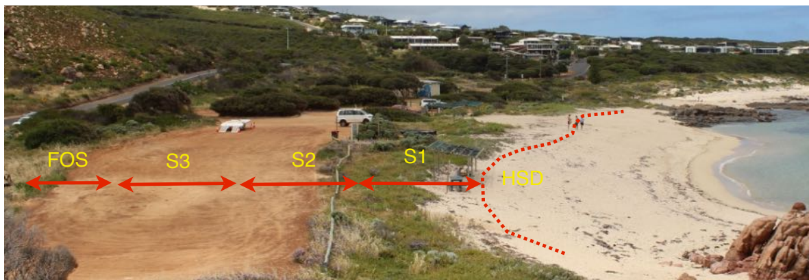
Figure 4-1 Representation of Planning Allowance for Coastal Processes on a Sandy Coast
