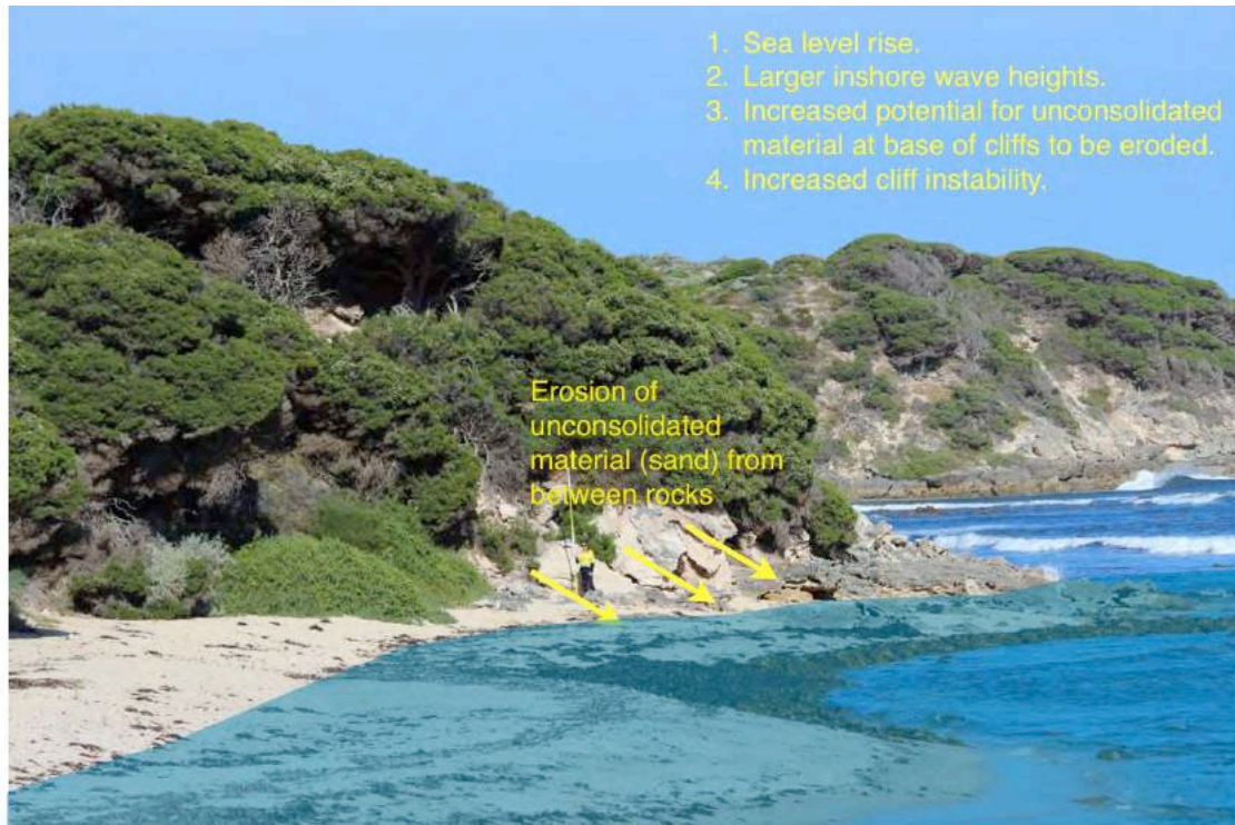
Figure 3.6 Concept for Weakly Lithified Sedimentary Rock Coast Response to Sea Level Rise
